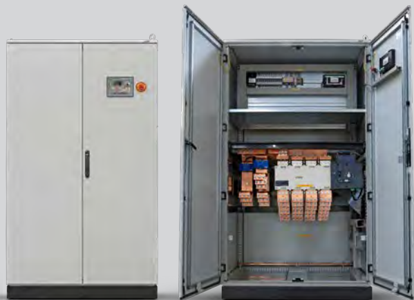
2500-3150 A Motorised 4-pole switch. Detection of mains failure and genset control. Emergency stop. Current and voltage measurement.
