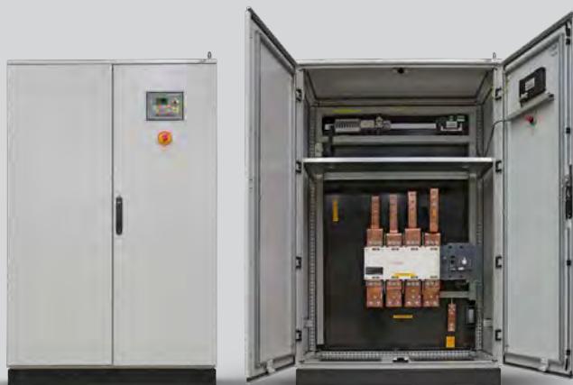
1600 A Motorised 4-pole switch. Detection of mains failure and genset control. Emergency stop. Current and voltage measurement.
