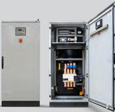
800 A Motorised 4-pole switch. Detection of mains failure and genset control. Emergency stop. Current and voltage measurement.
