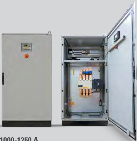
1000-1250 A Motorised 4-pole switch. Detection of mains failure and genset control. Emergency stop. Current and voltage measurement.
