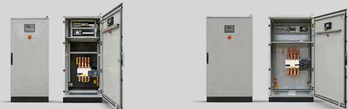
800 A Motorised 4-pole switch. Power failure detection. Emergency stop. Voltage measurement. 1000-1250 A Motorised 4-pole switch. Power failure detection. Emergency stop. Voltage measurement.
