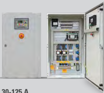
30-125 A 4-pole contactors. Detection of mains failure and genset control. Emergency stop. Current and voltage measurement.
