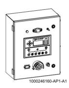
DSE-7320 is an advanced control module based on microprocessor, containing all necessary functions for protection of the genset and the breaker control. It can monitor the mains supply, and automatically start the engine when the mains is abnormal. Accurately measure various operational parameters and display all values and alarms information on the LCD. In addition, the control module can automatically shut down the engine and indicate the engine failure.
